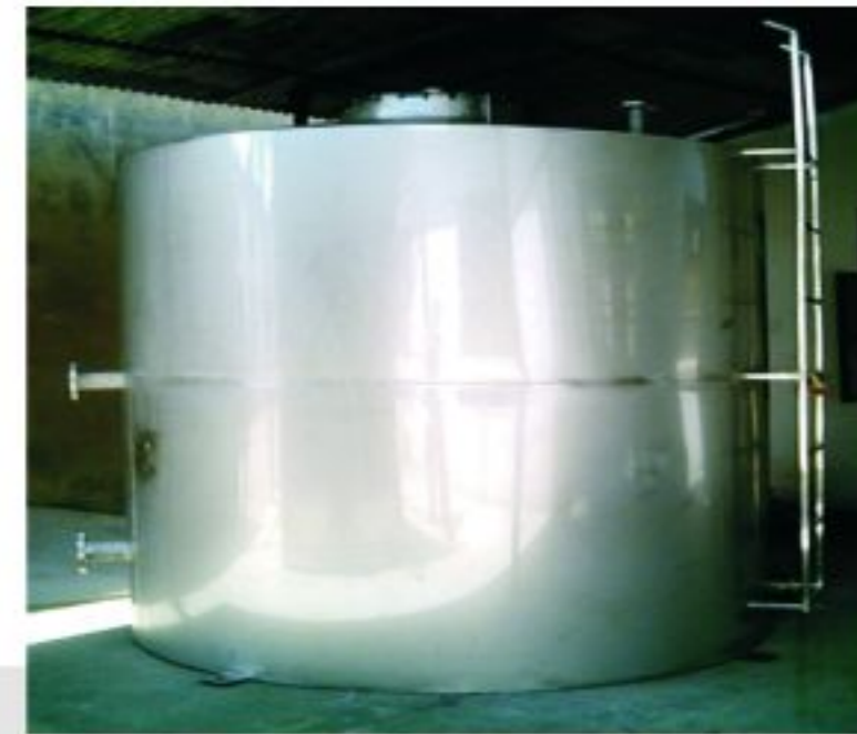
不锈钢储液罐 Stainless steel liquid storage tank
