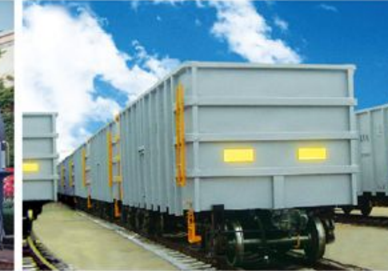
大秦铁路C80B不锈钢车 C80B stainless steel vehicle on Dalian-Qinhuangdao line
