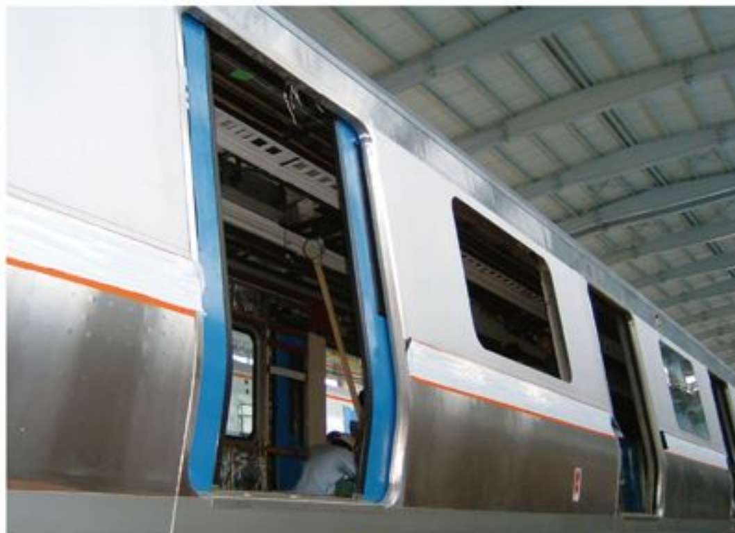
不锈钢地铁客车 (用钢00Cr17Ni7系列) Stainless steel subway passenger carriage (00Cr17Ni7 series)
