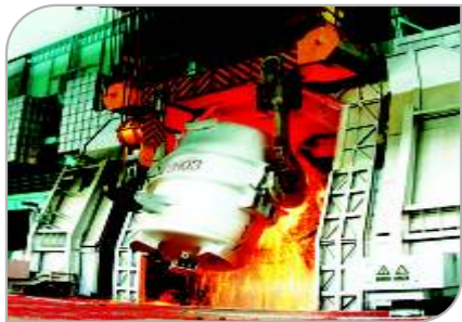
180吨顶底复吹脱磷转炉 180t Top and Bottom Blowing De-Phosphorus Converter
