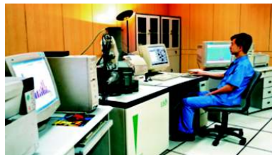
扫描电镜 Scanning Electron Microscope
